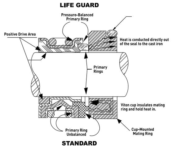
The drawing to the right represents a cross sectional view of a Life Guard Premium Silicon Carbide Seal (top) and a standard seal (bottom). There are three key differences shown in the drawing: material, mating rings and balance.
